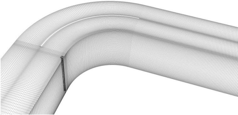
**Gambar 3.3** *Meshing square ducting* tampak isometri
