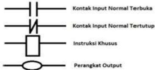
**Gambar 2.9** Simbol-simbol dasar ladder diagram
