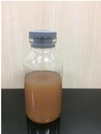
Gambar 4.2. Biodiesel + Metanol + Tween 80 1% +Span 80 1%
