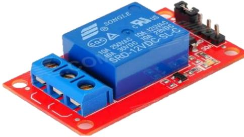
**Gambar 2.9** Modul Driver Relay
