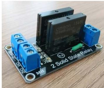
**Gambar 3.10** Modul *Solid State Relay*
