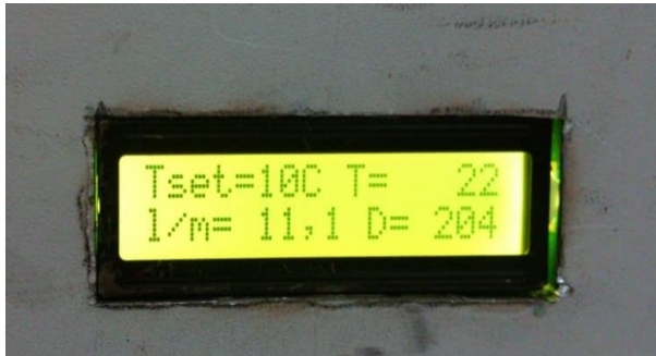
Gambar 4.3 Display LCD Kondisi Variable Speed Drive 80%
