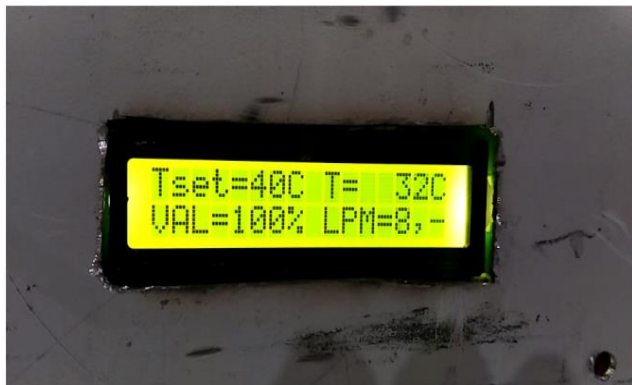
Gambar 4.4 Display LCD Posisi Bukaan Motor Operated Valve 100%
