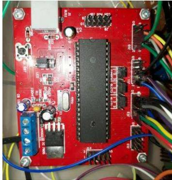
**Gambar 3.16** Sistem Minimum Atmega16
