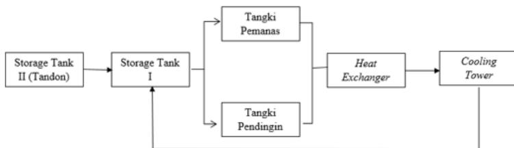
**Gambar 2.2** BFD Simulator Alat Penukar Panas
