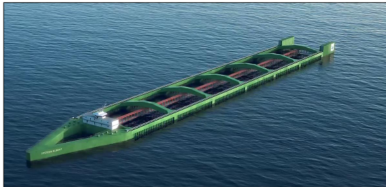
Gambar 2-6. Desain konseptual vessel-shaped fish farm . Sumber: (Hoiland 2017)
