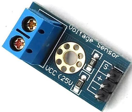
**Gambar C.1** *Voltage Sensor*
