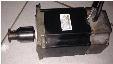
**Gambar 2.2** Generator ex motor servo AC
