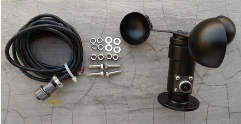
**Gambar D.1** *Universal Wind Speed Sensor*
