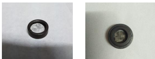
Gambar 4. 6 Gambar pellet HY sintesis (a)sebelum adsorpsi piridin (b)sesudah adsorpsi piridin
