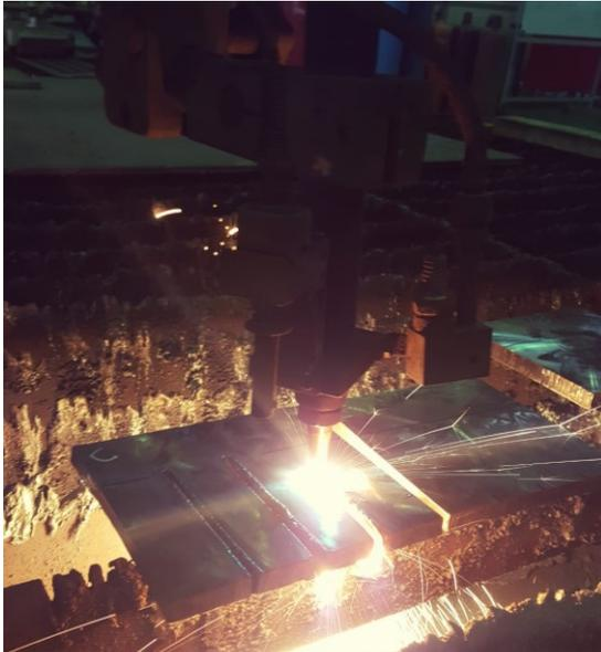
**Gambar 2. 6** Jenis Mesin Cutting Portable Single Cutting
