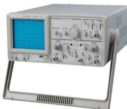
Gambar 2.23 Alat ukur *Cathoda Ray Oscilloscope* (CRO)
