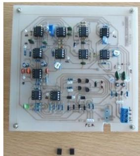
Gambar 4.9 Rangkaian *Electromyography* (EMG)
