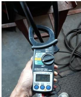
**Gambar 3.9** Tank Ampere
