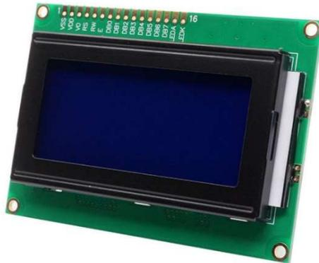
**Gambar 2.16** *Liquid Crystal Display*
