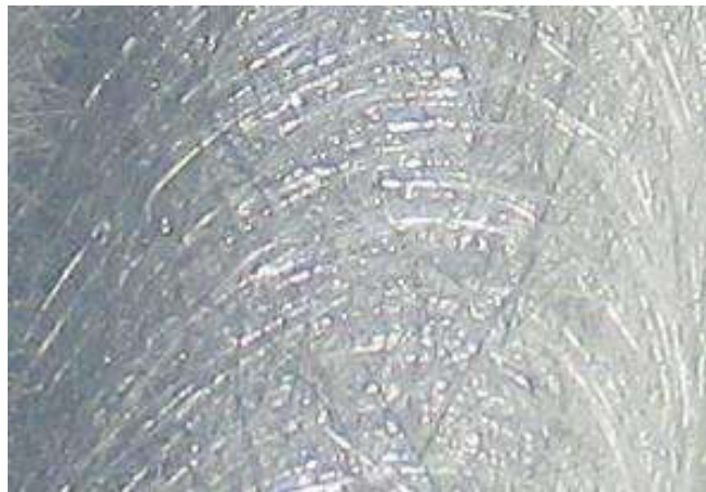
Gambar 2.5 Struktur Chopped Strand Mat (CSM)
