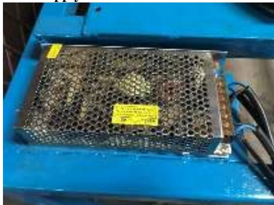
**Gambar 3.13** Power Supply 24 v
