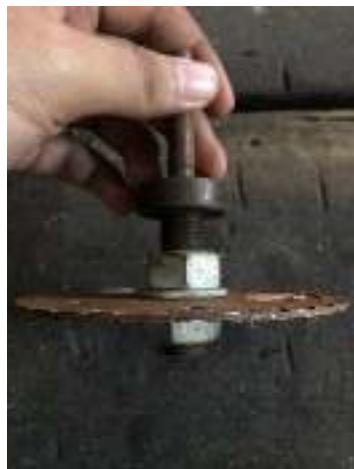
**Gambar 3.7** Metal-Bonded Grinding Wheel tampak samping
