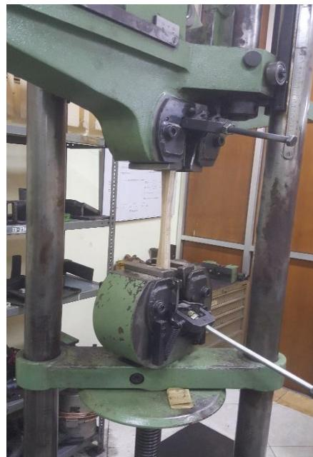
Gambar 3.5 Mesin UTM (*Universal Testing Machine*)
