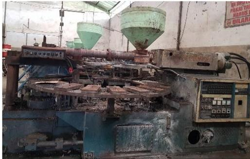
Gambar 3.2 Mesin Rotary Injection Molding
