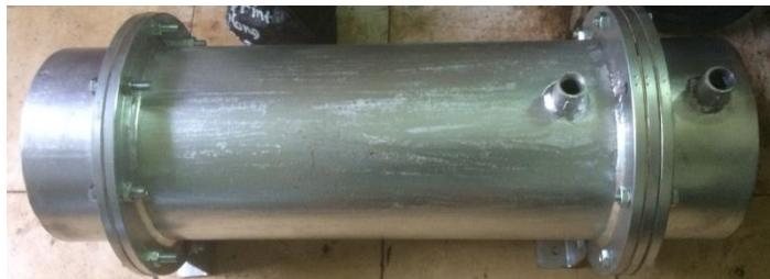
**Gambar 2 2** Tampilan Luar *Heat Exchanger Shell and Tube*
