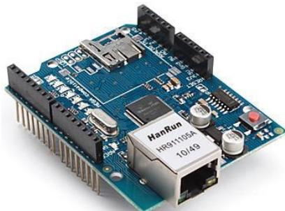
**Gambar 2.8** *Ethernet Shield*
