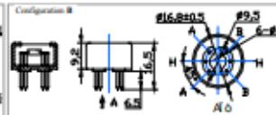
Structure and configuration of MQ-135 gas sensor is shown as Fig. 1 (Configuration A or B), sensor composed by micro Al<sub>2</sub>O<sub>3</sub> ceramic tube, Tin Dioxide (SnO<sub>2</sub>) sensitive layer, measuring electrode and heater are fixed into a crust made by plastic and stainless steel net. The heater provides necessary work conditions for work of sensitive
