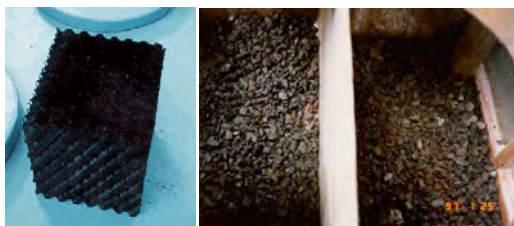
Gambar 2.5 Media Filter Sarang Tawon dan Batu Pecah
