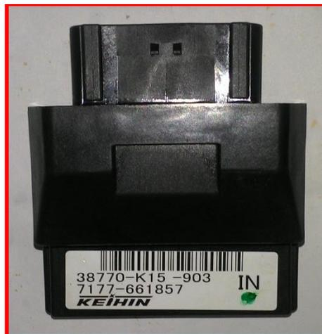
Gambar 3-6: ECU mesin standar
