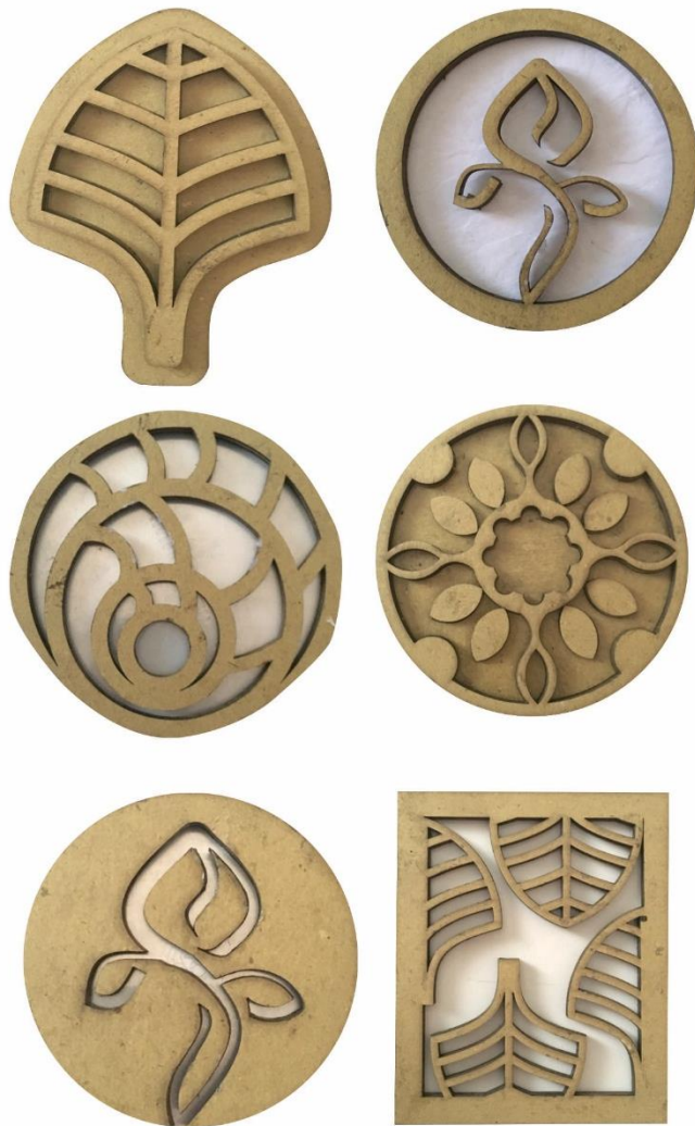
Gambar 4. 19 Hasil Laser cutting duplek (Sumber: Sitompul,2018)
