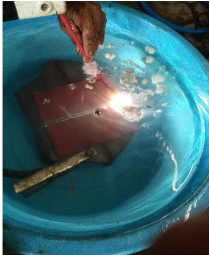
**Gambar 2.1** Proses Pengelasan Underwater
