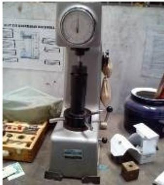
**Gambar 3.8** Alat Uji Kekerasan Rockwell
