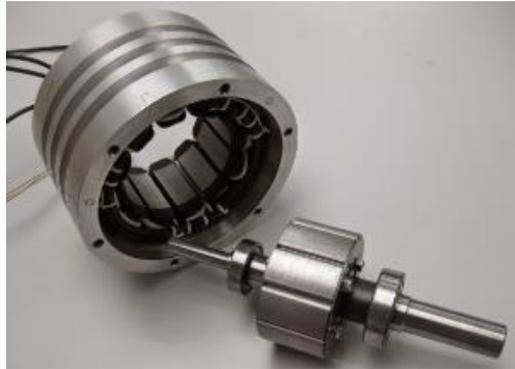
**Gambar 2.12** Bagian-bagian Motor PMAC
