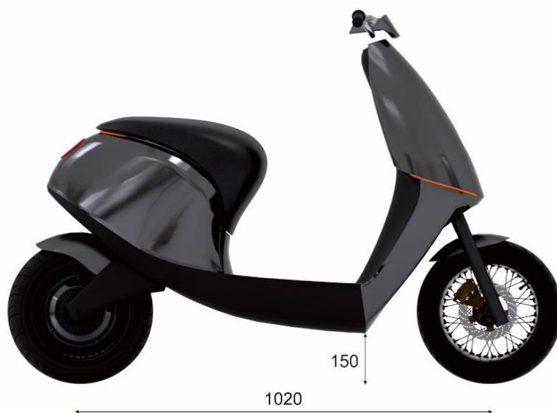
**Gambar 5.17** ground clearance dan wheel base
