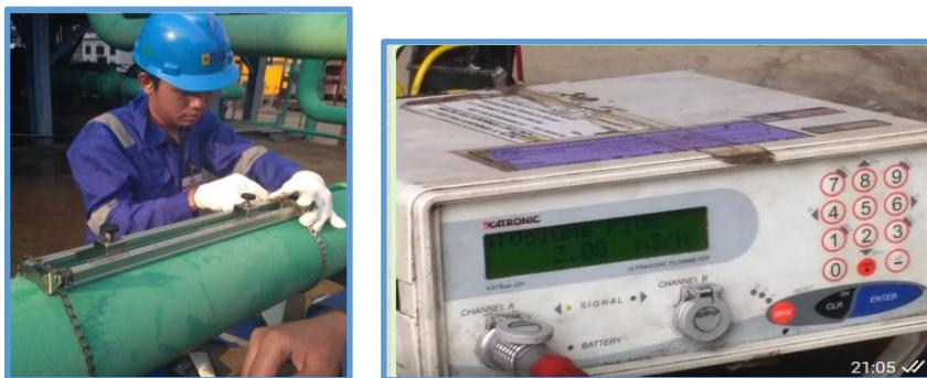
Gambar 2.15. Ultrasonic Flowmeter Katflow 220
