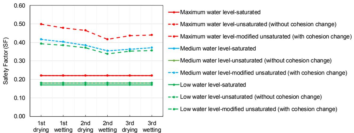
**Figure 9.10.** Curve of safety factor regarding saturated, unsaturated and modified-unsaturated slope stability
