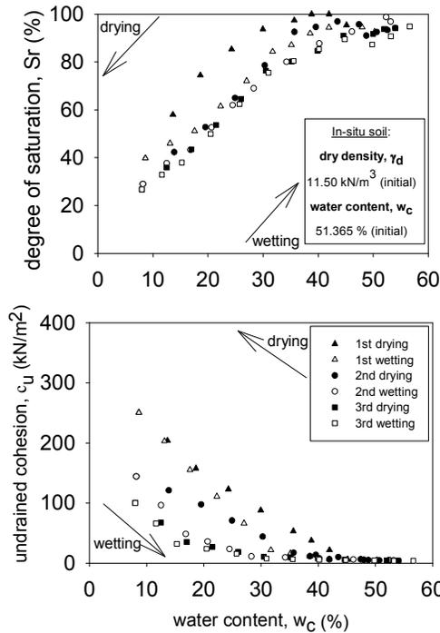
**Figure 6.10.** Mechanical soil properties change of in-situ soil due to cyclic drying-wetting test
