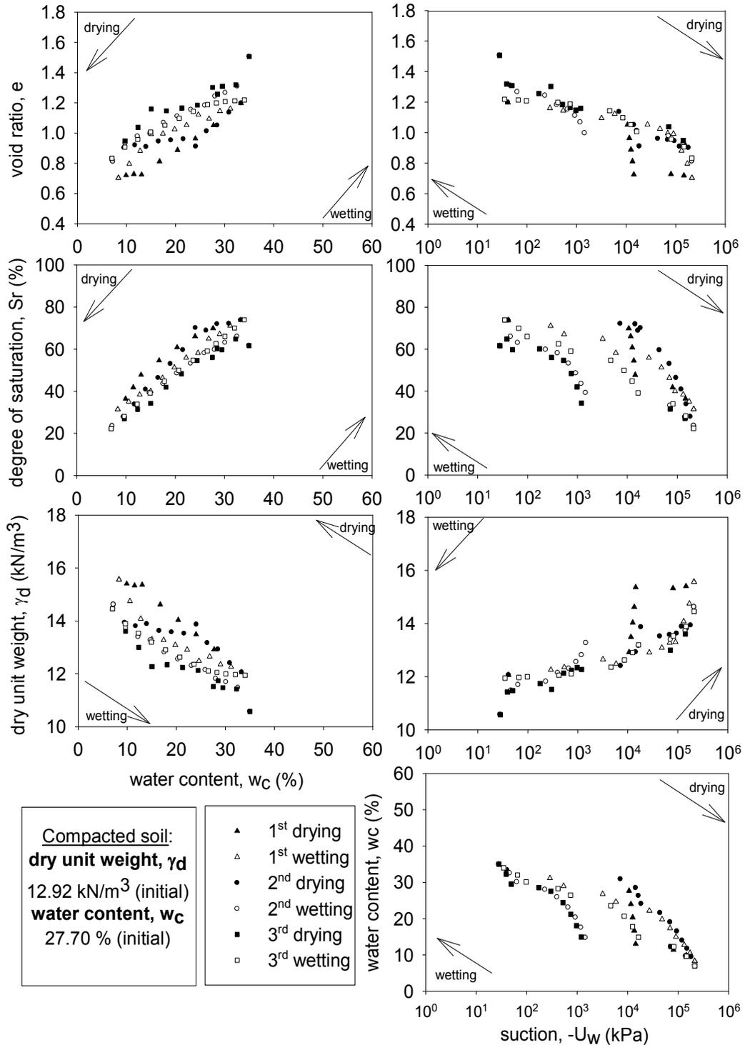
**Figure 6.11.** Physical soil properties change of fresh compacted soil due to cyclic drying-wetting test
