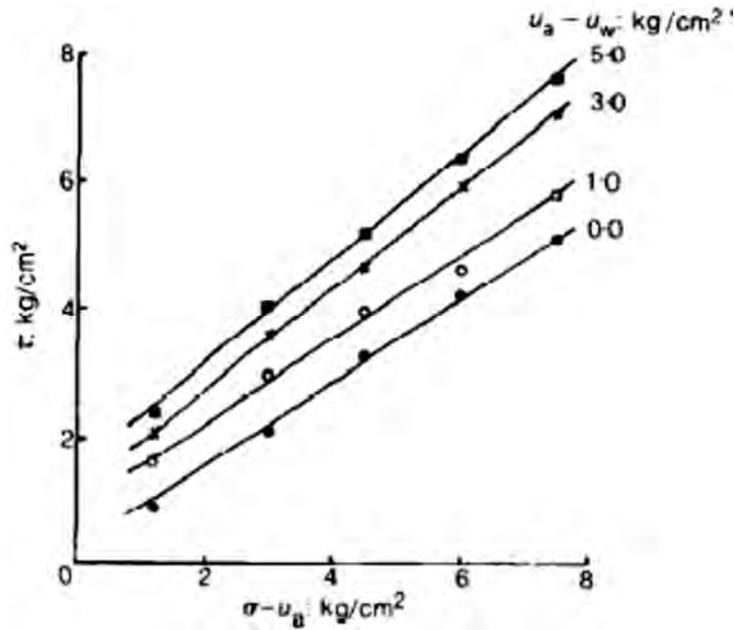
**Figure 3.11.** Shear strength data obtained for tests on Guadalix de la Sierra red clay in suction controlled direct shear tests (Escario and Sáez, 1986).
