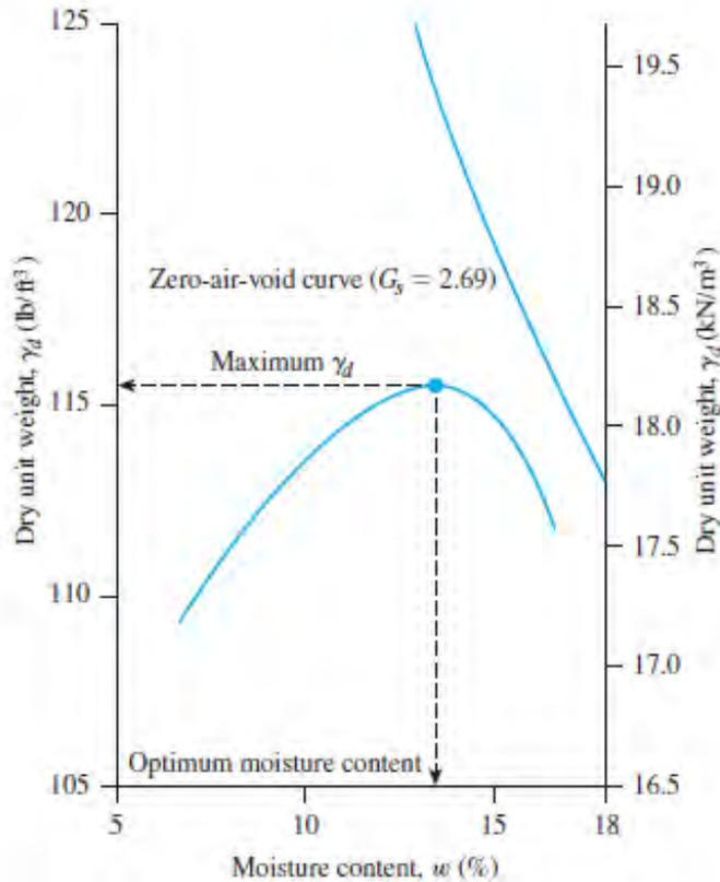
**Figure 3.4.** Standard Proctor compaction test results for a silty clay
