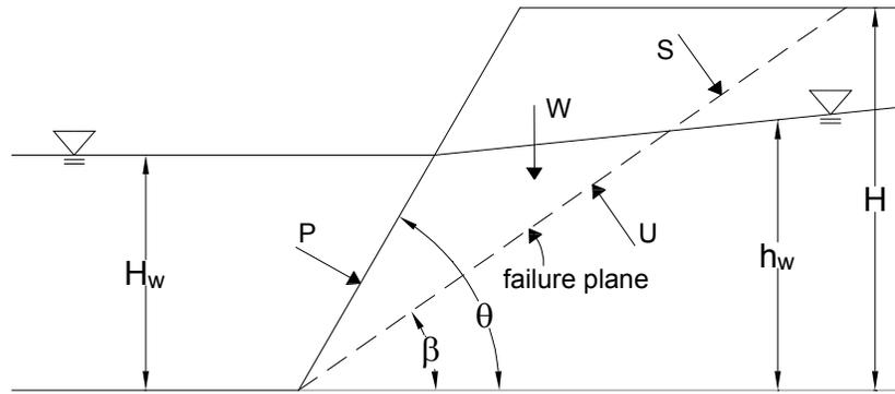
**Figure 9.4.** Forces on unsaturated slope stability (Chen, C.H. et al, 2017)
