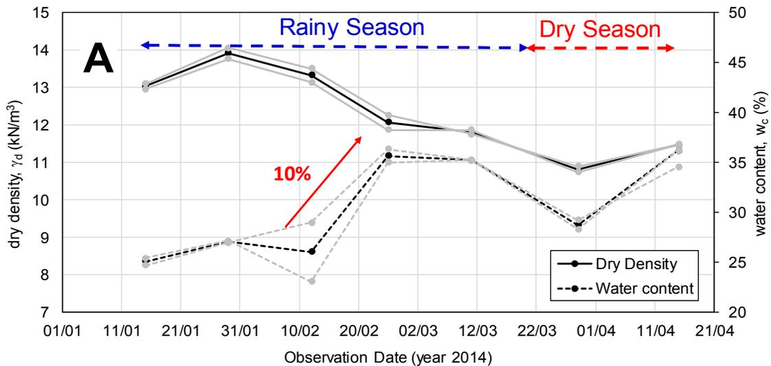
**Figure 6.2.** Relationship between dry density and water content during in-situ observation at section A
