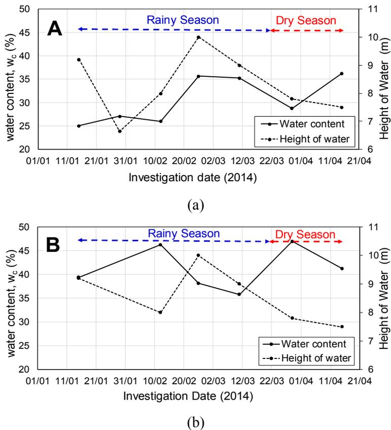
**Figure 6.1.** Water level fluctuation at (a) section A (upper part);(b) section B (lower part)
