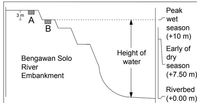
**Figure 5.2.** Detail of test location on river embankment
