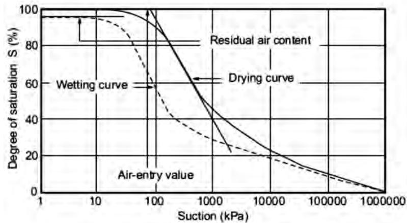
**Figure 3.7.** Typical soil-water characteristic curve features for the drying and wetting of a soil (Vanapalli et al, 1996).
