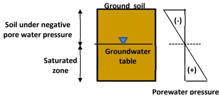
**Figure 3.5.** Soil profile under hydraulic condition (Fredlund, 2006)
