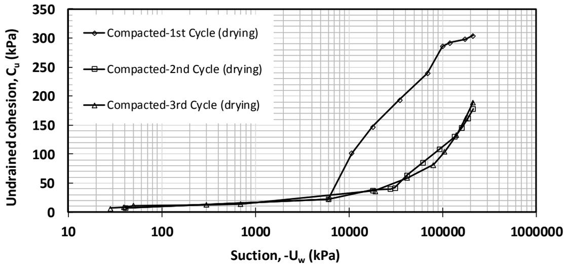
**Figure 9.7.** Relationship between suction ( $U_a - U_w$ ) and undrained cohesion ( $c_u$ ) along the drying test at 1<sup>st</sup>, 2<sup>nd</sup> and 3<sup>rd</sup> cycle
