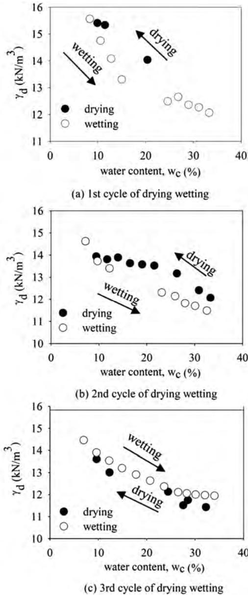
**Figure 8.1.** Comparison of water content ( $w_c$ ) and dry unit weight ( $\gamma_d$ ) due to cyclic drying-wetting
