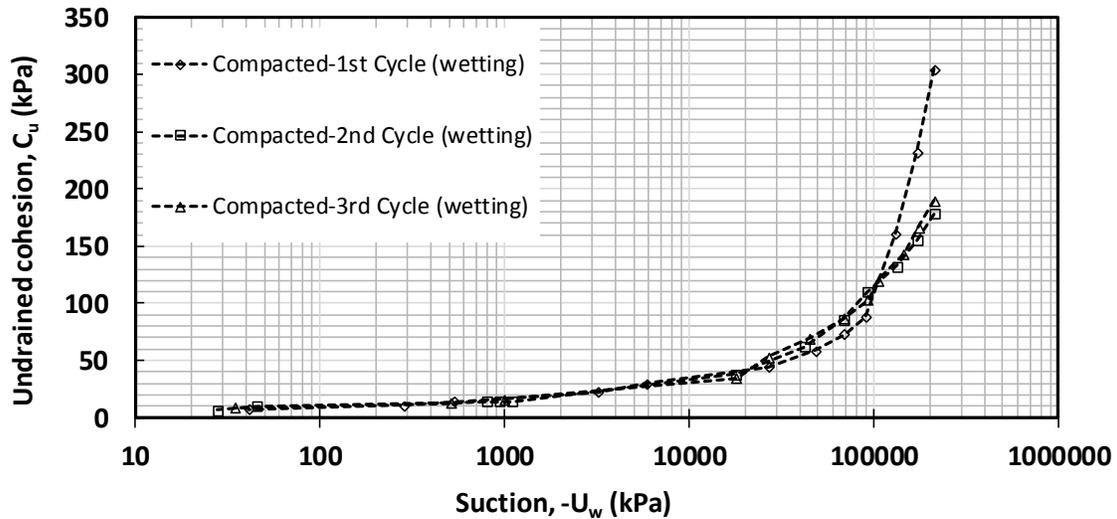
**Figure 9.8.** Relationship between suction ( $U_a - U_w$ ) and undrained cohesion ( $c_u$ ) along the wetting test at 1<sup>st</sup> cycle, 2<sup>nd</sup> and 3<sup>rd</sup> cycle
