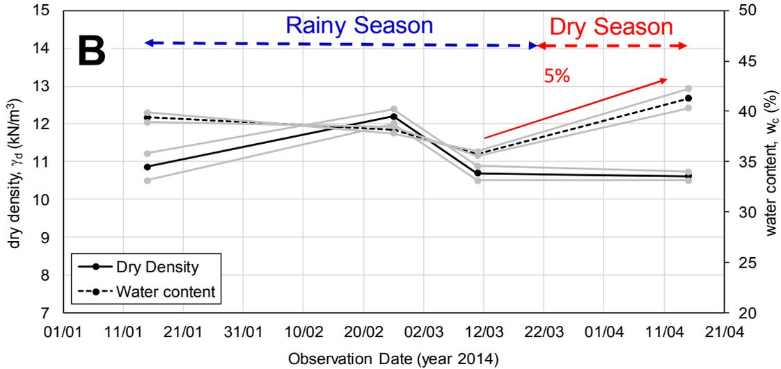
**Figure 6.3.** Relationship between dry density and water content during in-situ observation at section B
