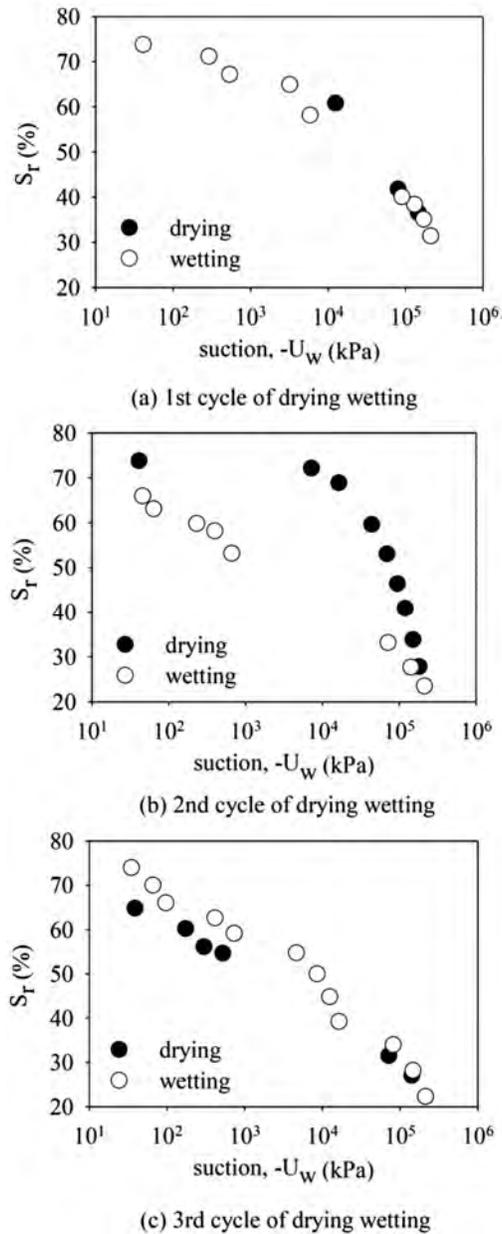
**Figure 8.2.** Comparison of suction ( $-U_w$ ) and saturation degree ( $S_r$ ) due to cyclic drying-wetting
