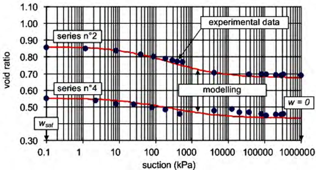
**Figure 3.8.** Void ratio versus suction from experimental data and modelling (Salager, S. et al, 2007)
