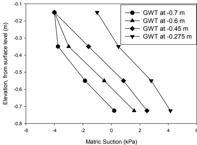
**Figure 7.1.** Pore-water pressure distribution during rising water table (Schnellman et al, 2010)
