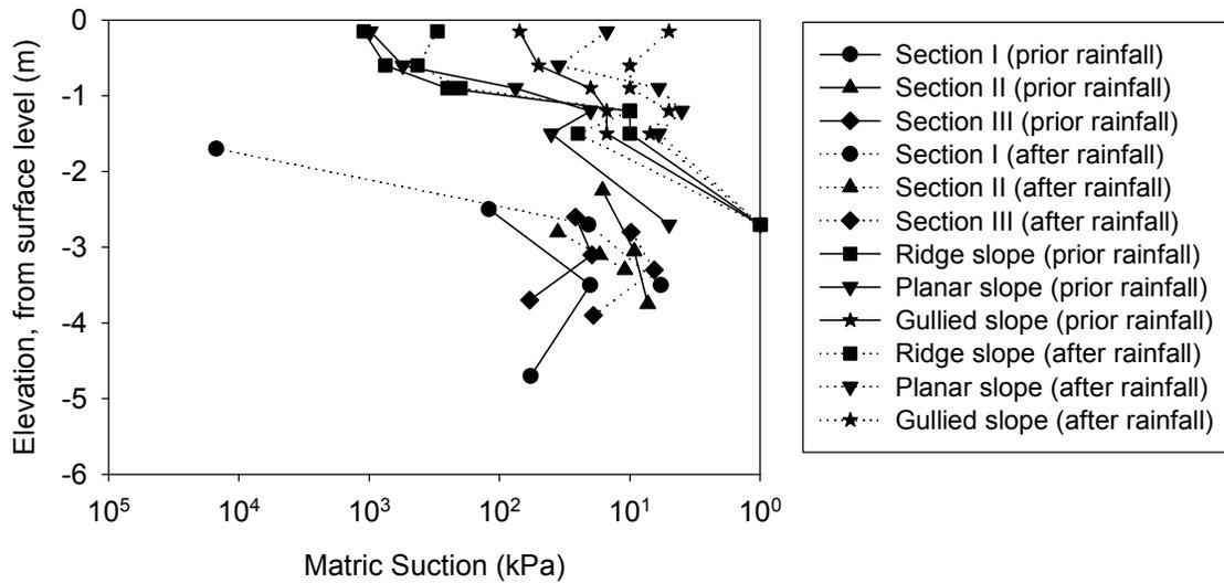
**Figure 7.4.** Suction profile at any elevation from monitoring result
