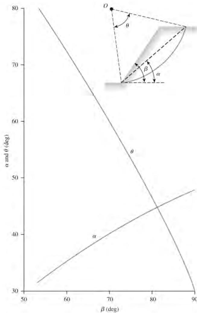
**Figure 9.5.** Location of the center of critical circles for  $\theta > 53^\circ$  (Das, B.M., 2010)
