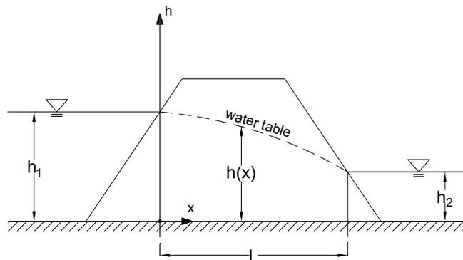
**Figure 9.1.** Water table through an isotropic earth embankment
