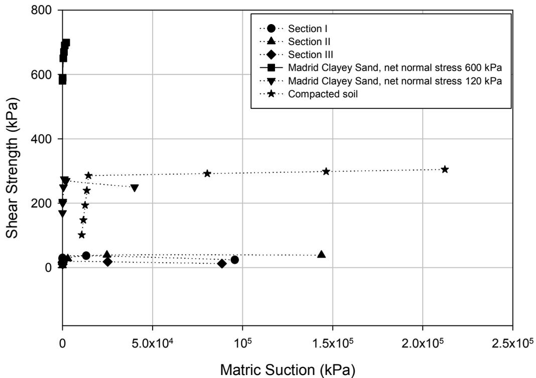
**Figure 7.3.** Relationship between matric suction and shear strength upon relevant studies
