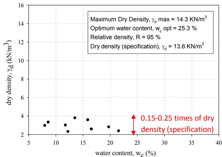
**Figure 2.3.** In-situ Investigation of Dry Density after 5 years construction, (Soemitro et al, 2007).
