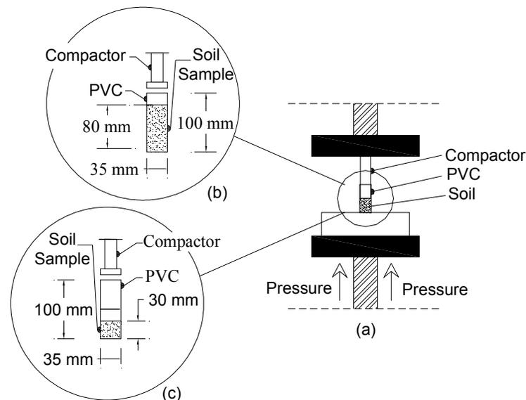
**Figure 5.3.** Remolding soil sample (a) compression machine; (b) soil sample dimension of unconfined compression test; (c) soil sample dimension of volumetric-gravimetric test
