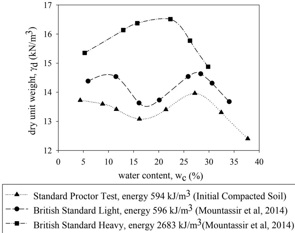
**Figure 7.7** Compaction test results in three different compaction energies
