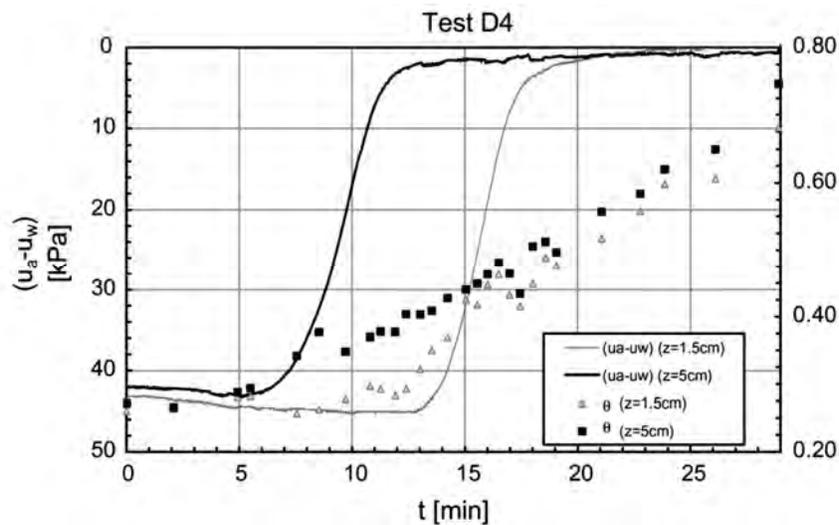
**Figure 3.2.** (a) instrumented flume; (b) matric suction (continuous and dashed lines) and volumetric water content (dots) time histories during infiltration experiments (Greco R. et al, 2010)
