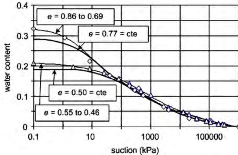
**Figure 3.9.** Comparison between different SWCC (Salager, S. et al, 2007)
