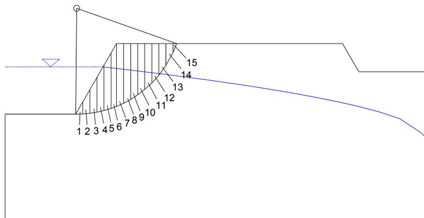
**Figure 9.9.** Method of slice during medium water level
