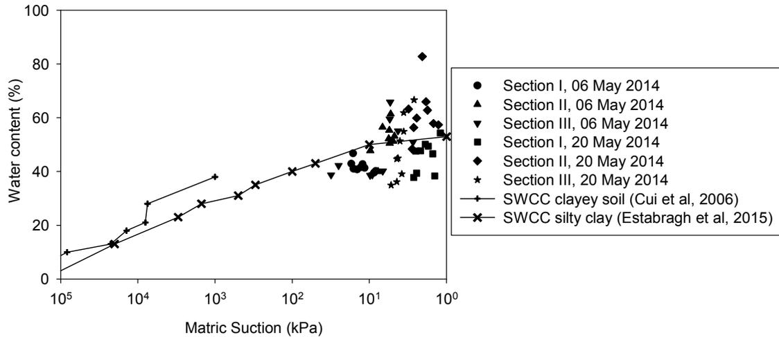
**Figure 7.6.** Comparison of soil water characteristics curve and suction monitoring result
