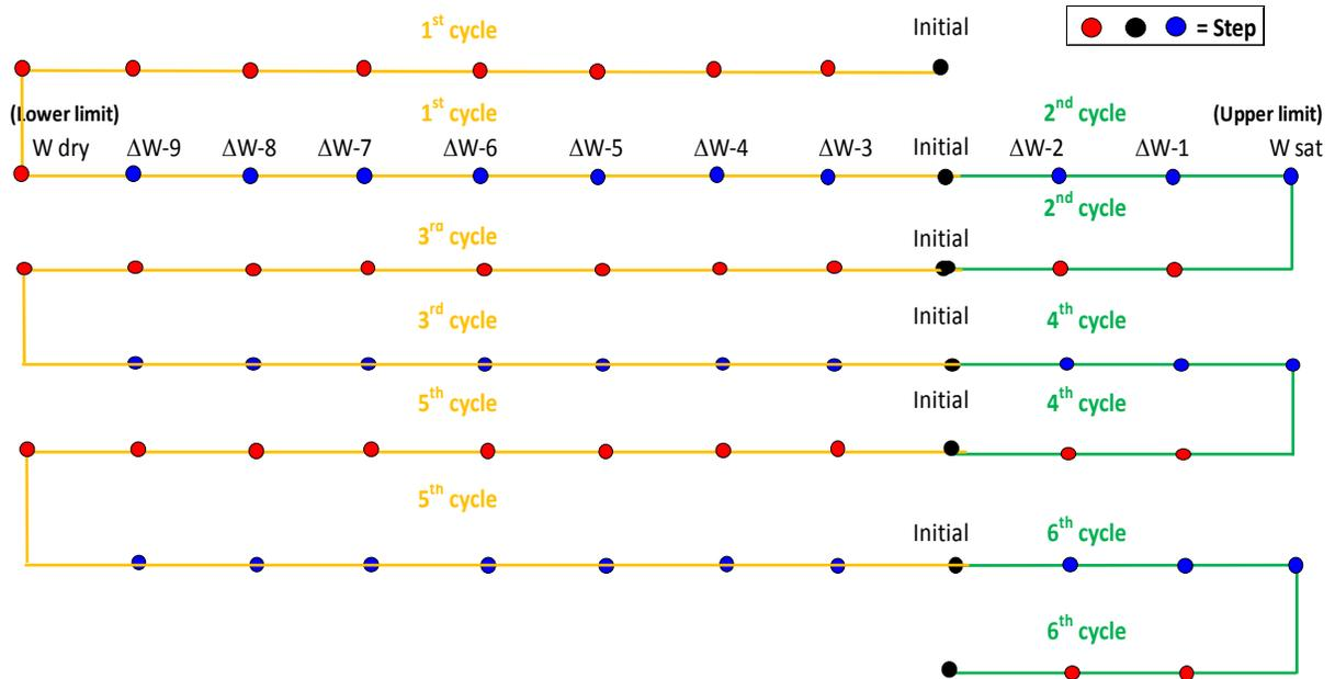
**Figure 3.6.** Drying-wetting process (Muntaha, 2013)
