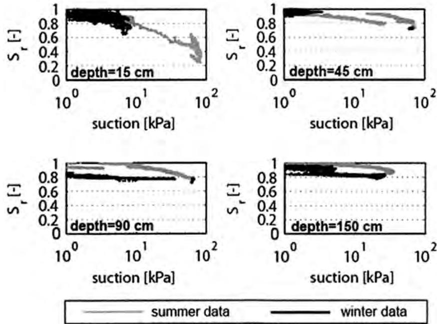
**Figure 3.1.** In-situ water retention curves in lower left test field
