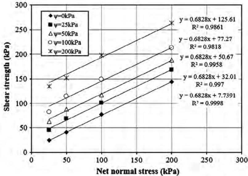
**Figure 3.3.** Failure envelopes due to different matric suctions of direct shear test (Zhou et al, 2016)
