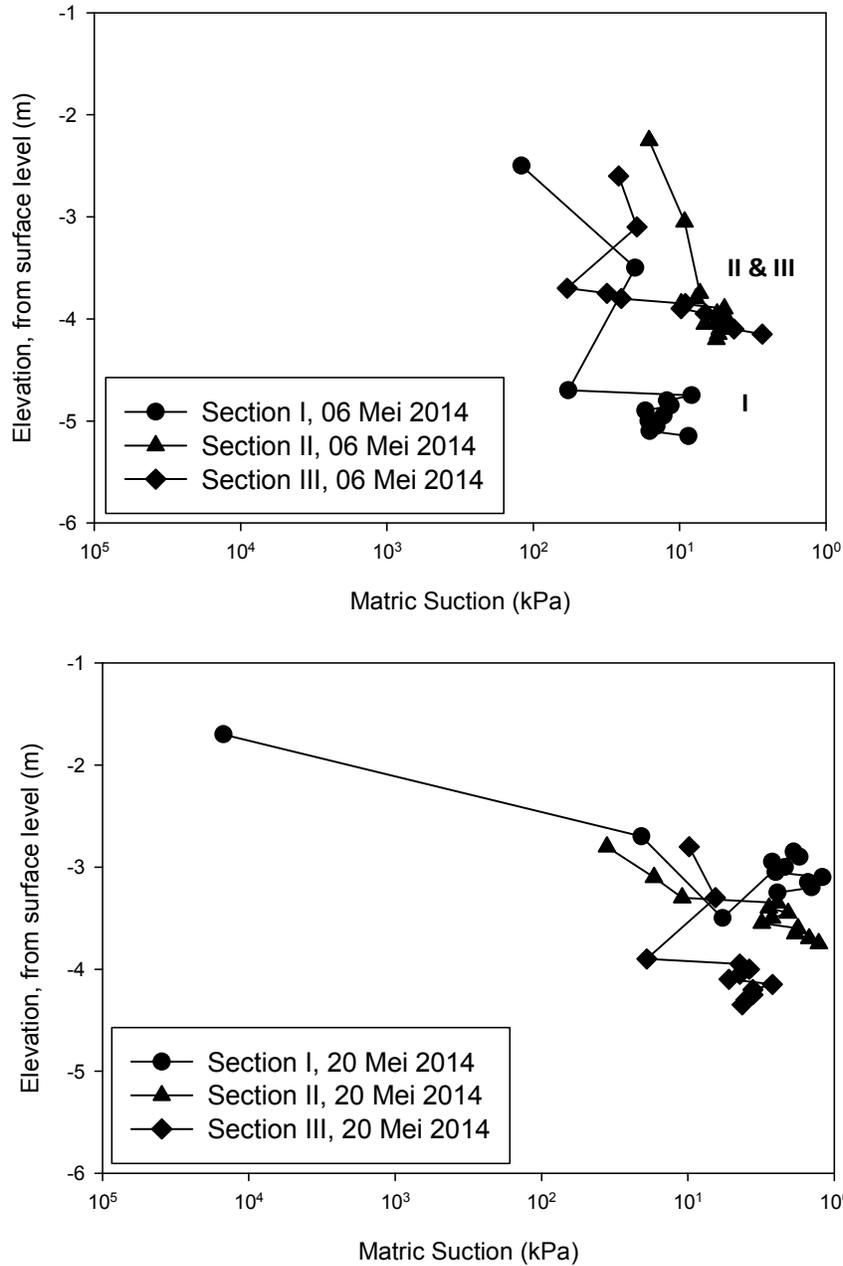
**Figure 7.2.** Suction in any observation depth at section I, II and III
