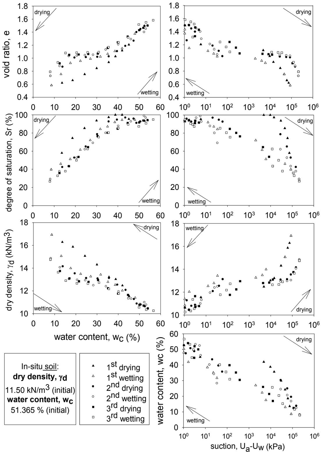
**Figure 6.9.** Physical soil properties change of in-situ soil due to cyclic drying-wetting test
