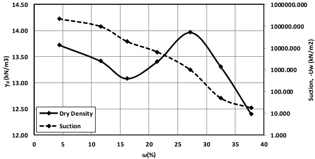
**Figure 6.7.** Laboratory compaction test results in three different compaction energies
