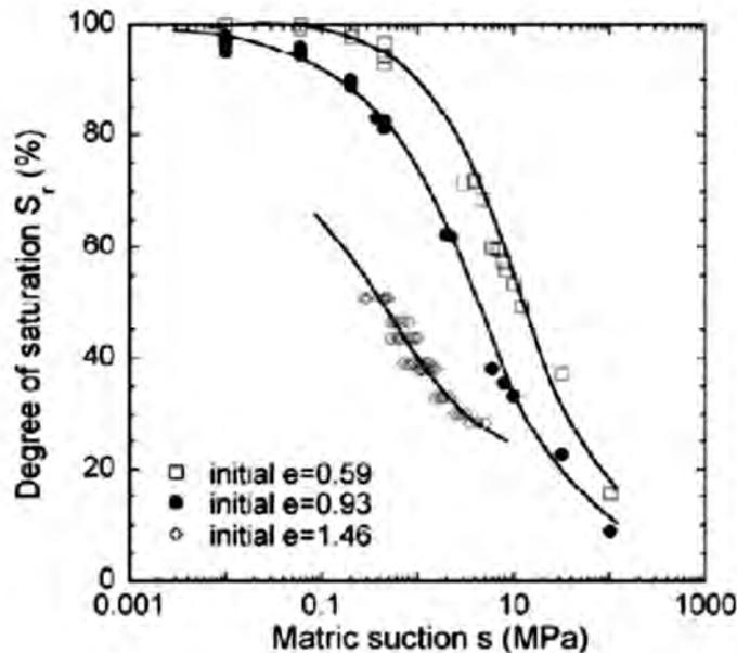
**Figure 3.10.** Influence of void ratio and structure on water retention behaviour of Boom clay (Nuth et al, 2008)
