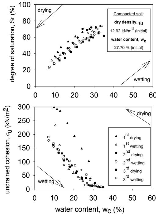
**Figure 6.12.** Mechanical soil properties change of fresh compacted soil due to cyclic drying-wetting test
