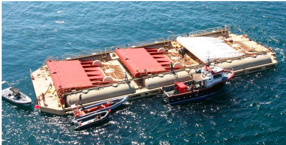
Gambar 2.5 OWS WaveRoller 100 Kw (Kasanen, 2015).
