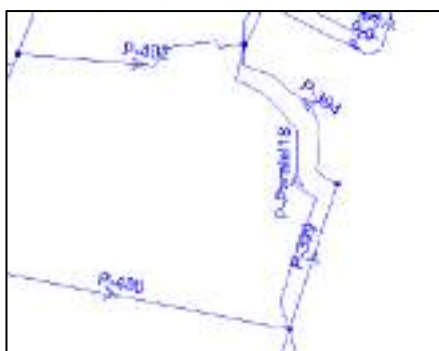
Gambar 5. 9F Penambahan Pipa Paralel 18
