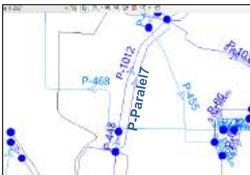
Gambar 5. 6F Penambahan Pipa Paralel 7
