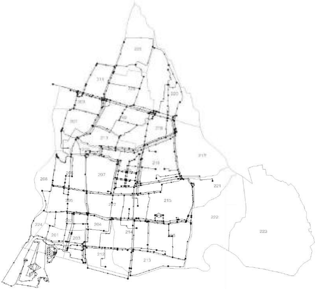
Gambar 5. 1 Model Jaringan Distribusi WaterCAD
