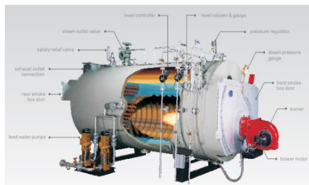
Gambar 2.3 Fire Tube Boiler [23]
