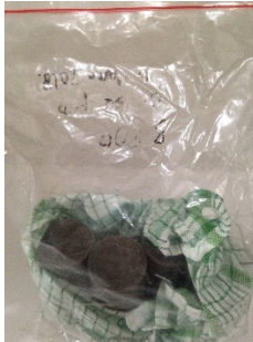
Gambar 3. 30 Perawatan moist curing benda uji silinder pasta (Sp)
