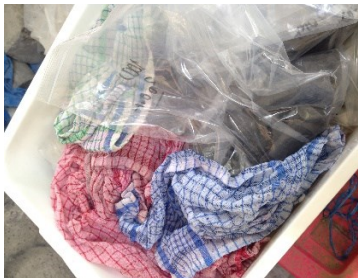
Gambar 3. 29 Perawatan moist curing benda uji silinder beton (Sn)
