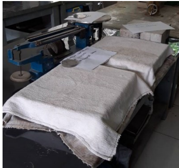
Gambar 3. 28 Perawatan moist curing benda uji balok beton (Bn)
