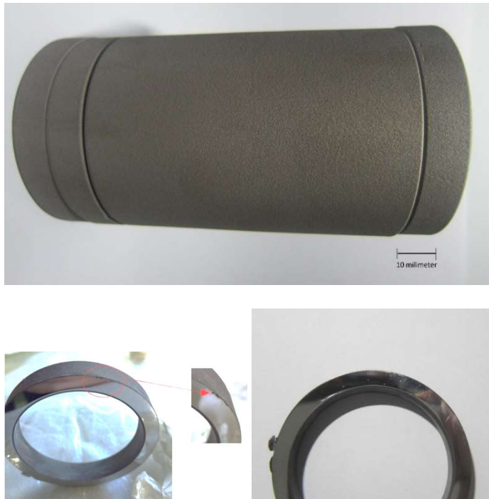
Gambar 4. 7 Visual coating NiCrBSi-30SiC 37 \mu\text{m}
