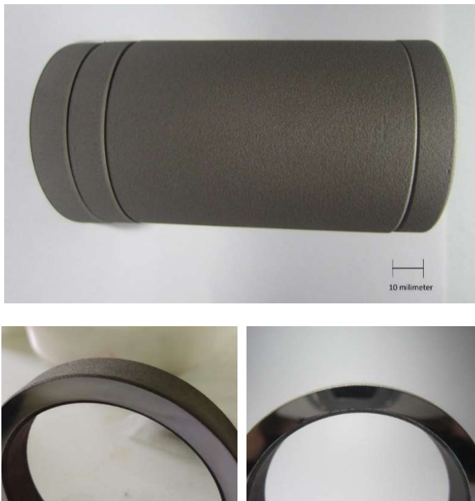
Gambar 4. 6 Foto Visual coating NiCrBSi-30SiC 50 \mu\text{m}
