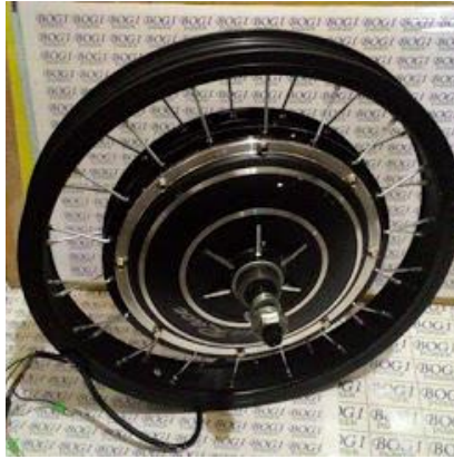
Lampiran Gambar 16 motor 48V 350W. ring roda 18"
