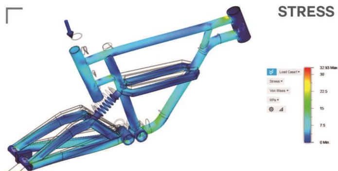
Gambar 37 Simulasi stress frame
