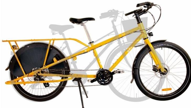
Gambar 4. 21 Perbedaan geometri longtail cargo bike
