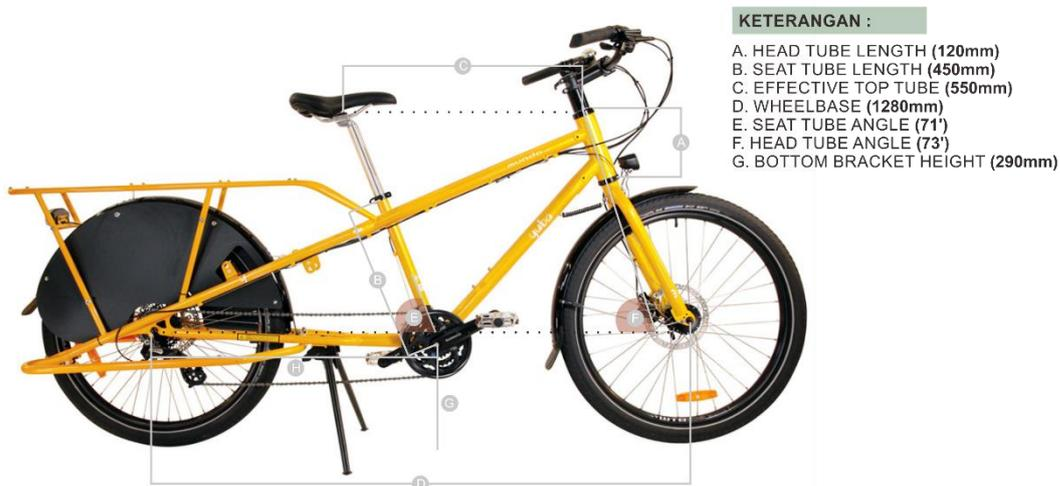
Gambar 4. 22 Geometri cargo bike YUBA MUNDO V
