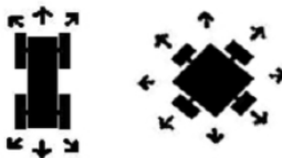
Gambar 2.1 Non-Holonomic Mobile Robot dan Holonomic Mobile Robot [2]
