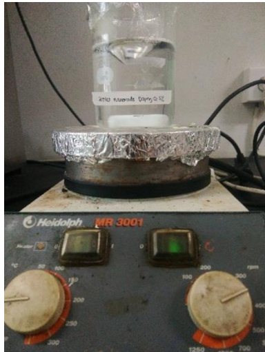
Proses stirrer larutan ZnO nanorods
