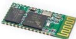
HC-05 module is an easy to use Bluetooth SPP (Serial Port Protocol) module, designed for transparent wireless serial connection setup.
