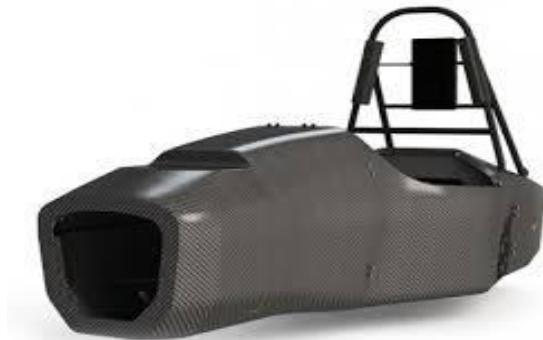
*Gambar 2.6 Chassis Monocoque*
