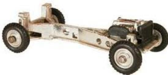
**Gambar 2.7 Chassis Backbone**
