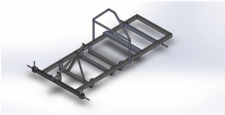
**Gambar 2.2 Design Chassis Nogogeni V**
