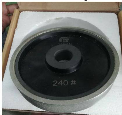
**Gambar 3.9** Diamond Abrasive Grinding Wheel
