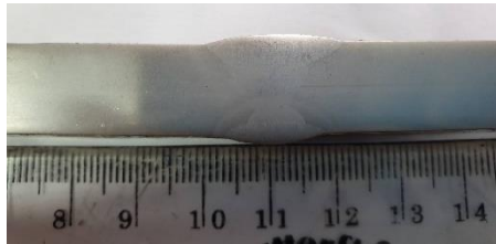
Gambar 4.8 Lebar HAZ Arus 170A
