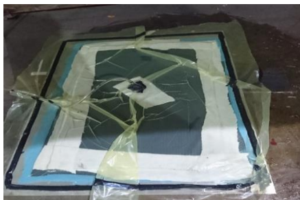
Gambar 3.22 composite sandwich sebelum proses out-of-autoclave
