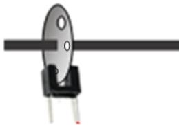
**Gambar 2. 9** *Rotary Encoder* [1]
