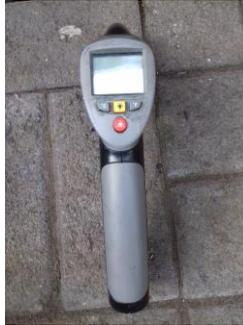
**Gambar 3.10 Infrared thermometer**
