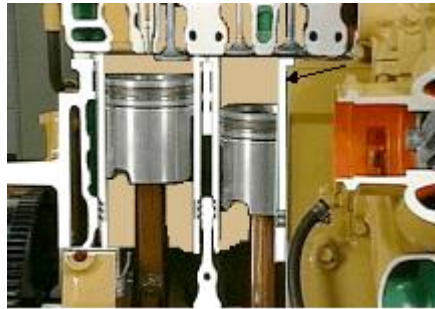
Gambar 2. 16 Cylinder Liner (“Modul Training Basic Mechanic” PT. Vale Indonesia, Tbk, Sorowako 2017)
