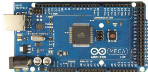
Gambar 2.1 Tampilan Depan Arduino Mega 2560 [5]
