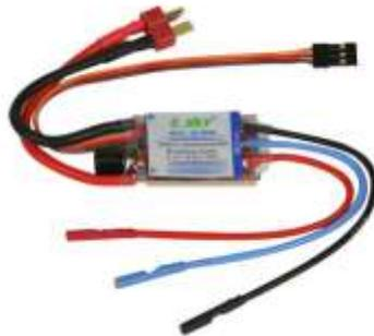
**Gambar 2.5** ESC (*Electronic Speed Controller*)[1]
