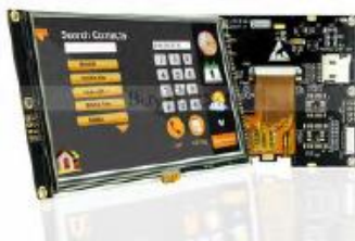
← ER-TFTM050-2 with Capacitive Touch Panel
