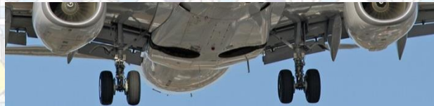
Figure 1.1. The Main Landing Gear in B737-800NG
