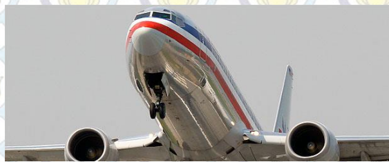
Figure 1.2 The Nose Landing Gear in B737-800NG
