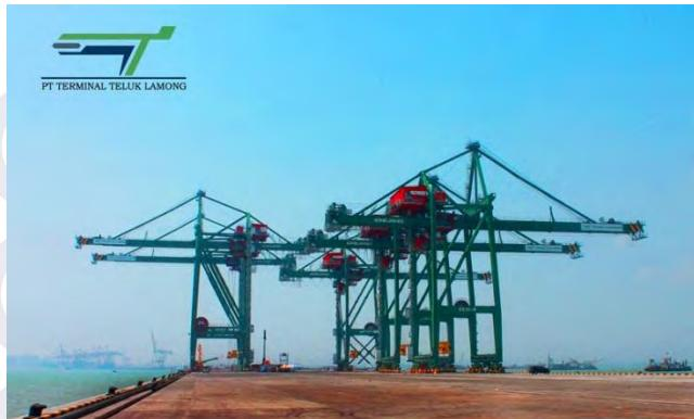
Gambar 2.3 *Ship to Shore Crane (STS)*
